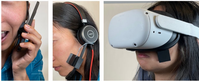
Figure 13: Mock-ups of Füpop electronics integrated into a cell phone, an audio headset, and a head-mounted display.
