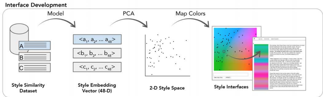
Figure 3. From left: Style comparisons from the collected dataset are used to train a predictive model, which learns a high-dimensional vector embedding associated with how people perceive style. The embedding is projected to 2 dimensions using principal component analysis (PCA). By mapping a color space to the 2D projection, the style of text excerpts can be associated with a color, and used to create interactive experiences (Left Interface: Explorer; Right Interface: Editor).
